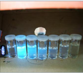
Fluorescence occurs when UV absorption and visible light emission interact. The picture on the left shows the blue fluoresces of horse chestnut extract on the left side and ash extract on the right side. The blue fluorescence in the second picture diminishes from one snap capped vial to the next. The first snap-capped vial serves as a blank containing water.
